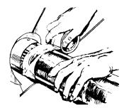
Attach exhaust duct to each dryer duct. Then connect exhaust ducts to exhaust hoods or main exhaust. Use duct tape to seal all joints.
